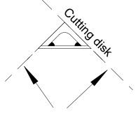
Cut near the joint and grind flat
