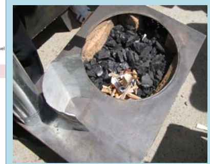
Simple change of firing technique gives much improvement in emission
