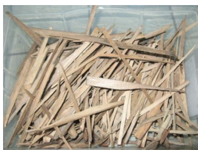
Figure 6: Woodchips for WBT and AWBT starting phase (average size: 0.3x0.3x10cm)
