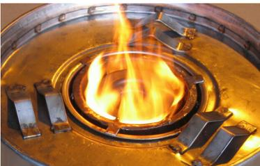
When the paraffin enters the hot heater pipe, it will make a rushing sound as the gas leaves the jet and burns under the bluff plate. During this time the heater pipe continues to increase in temperature and the flame is not stable. If you open the fuel control valve at just the right time, the fire will not smoke at all.
