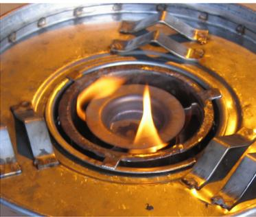
The methylated spirits will burn well and will heat up the heater pipe to a temperature that will boil the paraffin into a gas. If you look into the bottom of the combustion chamber you will see the spirits burning in the centre. A few moments before the flame is going to go out, open the fuel control valve about half way.
