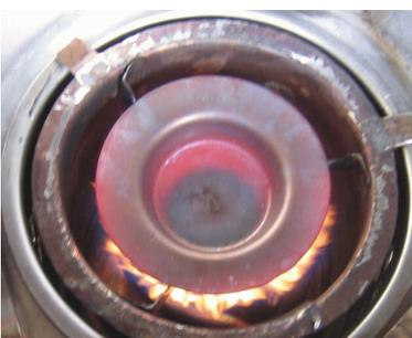
Adjust the fuel control valve so that the flame is not whooshing. At high heat there is can be a tendency to puff or flash-flame. The flame might blow itself out. Turn the valve more closed until the flame is steady. The picture shows the stove running at a low heat. At all times there should be a 'roaring' sound from the flames. Closing the valve too much kills the sound and makes smoke.
