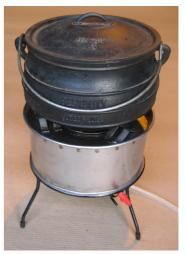
**Lastly:** to turn off the stove, close the fuel control valve and blow out the thin orange flame (or it makes a little bit of smoke).
